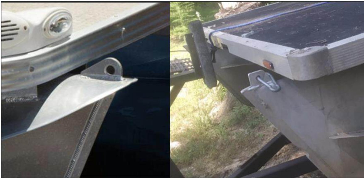
Figures 2 and 3. Front Hook Located in the Corner of the Pontoon
