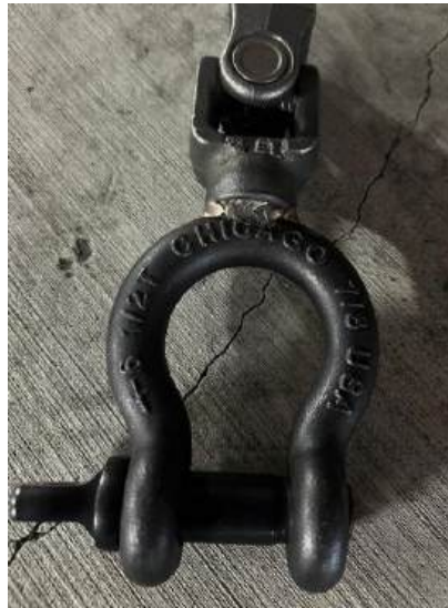
Figure 39. D-Shackle welded to Universal Joint
