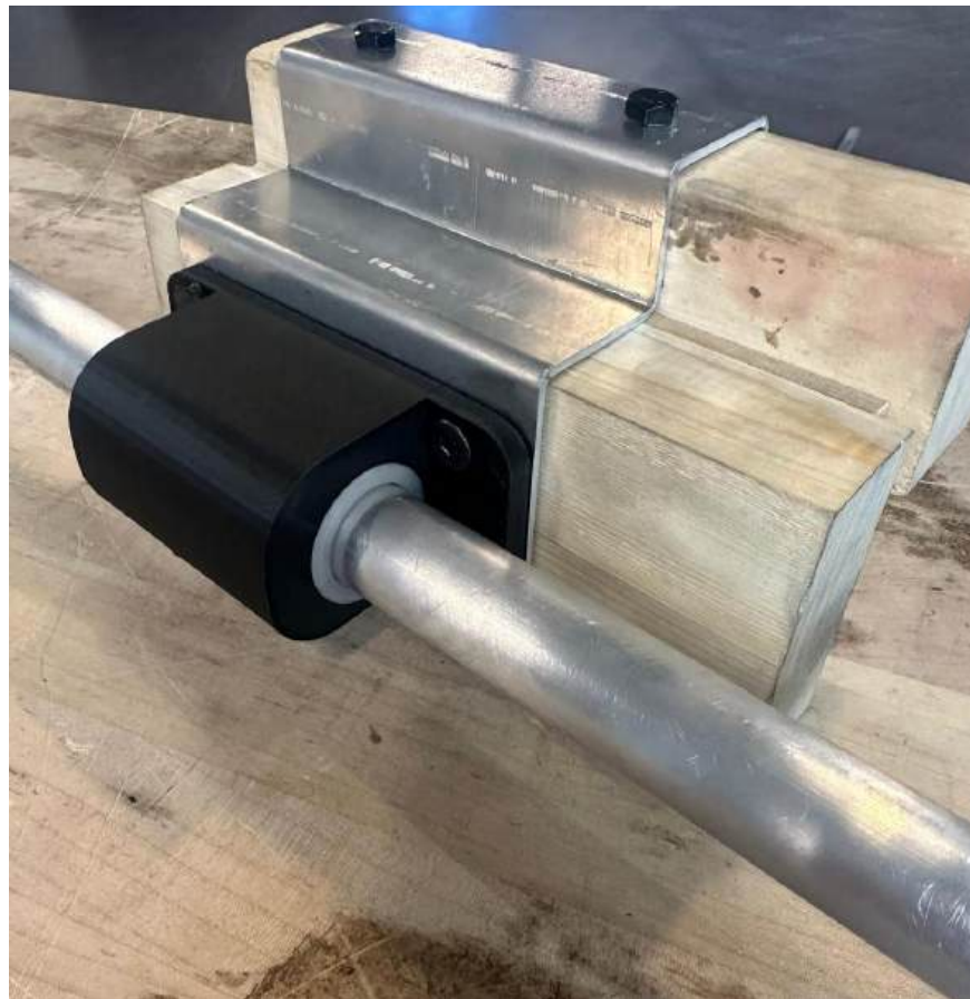
Figure 41. Pontoon Back Connection
